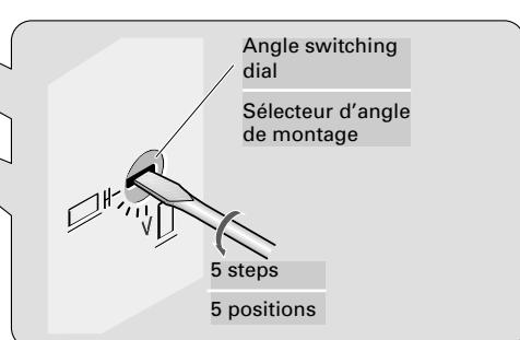
The angle switching dial must be set on both sides of the player to the same position.
